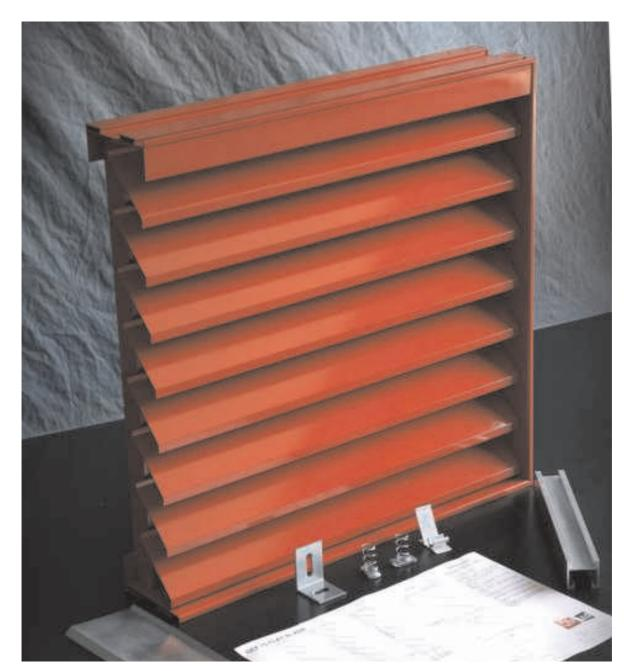
Single bank extruded aluminium flat blade louvre pitched at 75mm- the standard commercial louvre blade pitch to be used where sharp lines and flat surfaces form part of the architectural design. Used for general applications where good airflow is required and reasonable weathering is achieved except under severe conditions.
