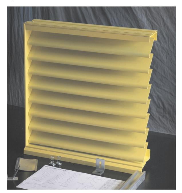
Single bank extruded aluminium curved blade louvre pitched at 75mm- the standard commercial louvre blade pitch with an aerodynamic curved profile for smooth airflow. Used for general applications where good airflow is required and reasonable weathering is achieved except under severe conditions.
