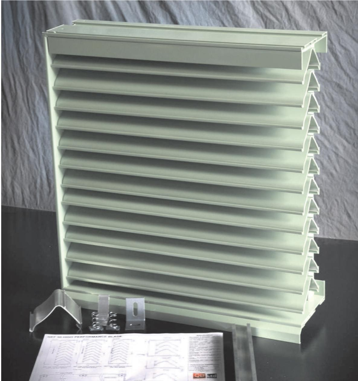
High Performance double pass extruded aluminium curved blade louvre pitched at 50mm. Designed with Irish climatic conditions in mind, to minimise rain penetration whilst maintaining a good airflow. Tested at BSRIA to Class A3 up to 2.4 m/s face velocity; the top performing horizontal louvre tested to date. This louvre also has the benefit of non vision through the louvre viewed from any angle.
