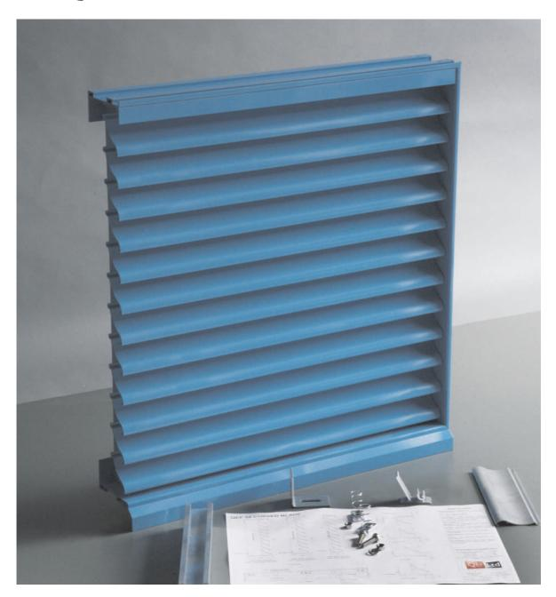
QEF 50 Curved Blade single bank extruded aluminium louvre pitched at 50mm. This is a scaled down version of the 75 Curved Blade, resulting in an improvement in the weathering performance due to smaller blade gap and limited reduction in the airflow. The aerodynamic curved profile and reduced pitch present an aesthetically pleasing louvre for architectural facades. The smaller louvre depth is of benefit where space is limited.
