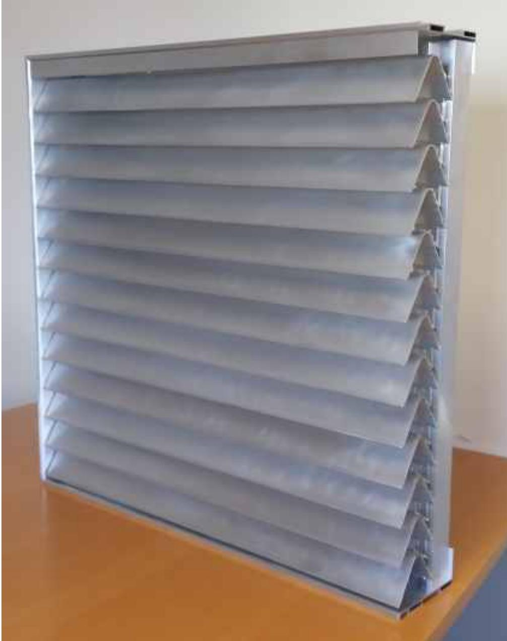
Double bank extruded aluminium curved blade louvre pitched at 50mm. The double pass blade design results in an improvement in the weathering performance to class A for velocities up to 1.0m/s face.
