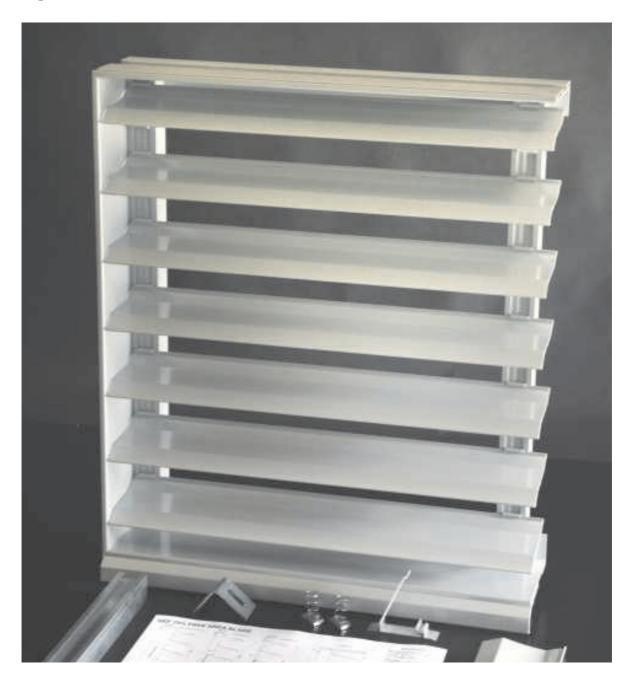
Single bank extruded aluminium flat blade louvre pitched at 100mm, designed specifically for where a high open area is required and weatherability is not an issue. Typical applications include basement car parks with limited wall space for louvre openings and a need to achieve specific free areas to meet the fire regulations.
