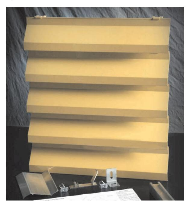
Single bank extruded aluminium 'zed' shaped blade louvre pitched at 140mm, designed specifically for use as an external plant screen where weathering is not required. The large louvre blade profile and increased spanning capability result in an economical solution for applications where large areas need to be screened; louvre blades can be inverted where the predominant view is from a low level.
